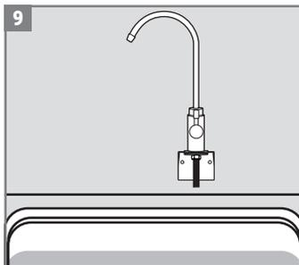
In case of wall-mounted installation of the faucet use the „L“ connector to fix the faucet similar to the descriptions in picture 11-12.
