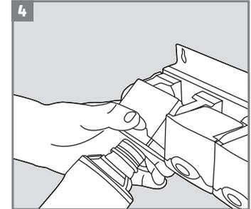
Press the push button and rotate the filter to eject.
