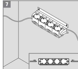
7 Insert the plastic tube and connect the adapter on the wall.
