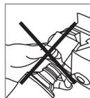
Never use the PUSH button for filter replacement during water flow. The equipment may break down due to high pressure. For filter exchange close the diverter valve.
