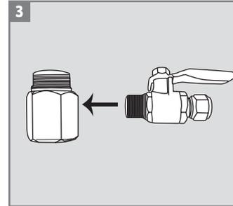
3 Connect the diverter ball valve with the nipple (use teflon-tape).
