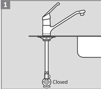
1 Lock the stop valve of the cold water supply line.
