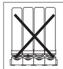
Please install the filter upright. In case of moving or raising the filter make sure that the filter stays upright.
