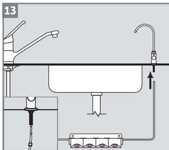
Connect the outlet tube with the drinking water faucet connector.
