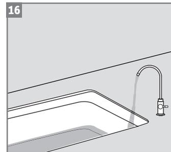
If there is no installation mistake or leakage keep the faucet open for 10 minutes to bring rest particles and air out of the unit.
