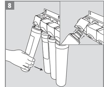
8 Bring the adapter in upward position and insert the filter. A loud "click" will signal that the filter is attached properly. Bring the filter back in the normal position.
