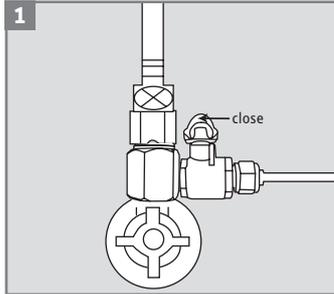
Close the diverter valve under the sink.
