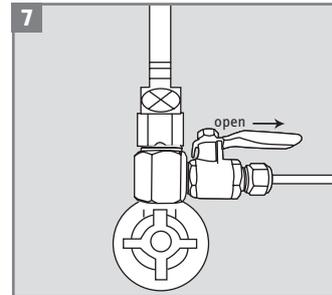
Open the diverter valve under the sink slowly. Check the whole system for water leakages.
