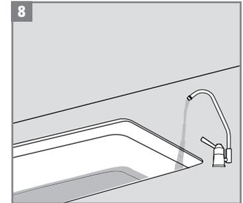
If there is no installation mistake or leakage keep the faucet open for 10 minutes to bring residual particles and air out of the unit.
