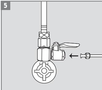
5 Cut the plastic tube in 2 pieces. Connect the inlet tube and tighten the tube with the cap.
