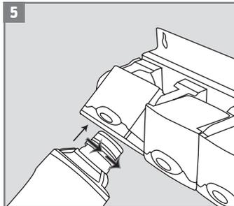
Remove the cap of the new filter and insert in the head connector. A "click" will signal that the filter cartridge is connected properly.
