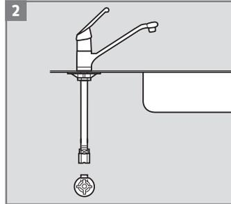
2 Detach the metal hose from the cold water supply under the sink.
