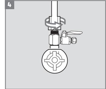
4 Assemble the ball valve and nipple to the water supply. Re-attach the metal hose.
