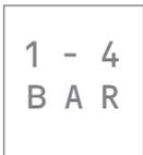
To reach an optimized and satisfying filter result the water filter should only be installed in houses with a pipe pressure between 1 and 4 bar.
