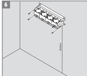
6 Select a proper place under the sink that has at least 25 cm (10") / 30 cm (13") from the floor to allow to insert the cartridges easily. Make holes into the wall to fix the filter adapter under the sink.
