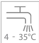
The filter can only be installed to the cold water supply with a water temperature between 4 and 35°C.
