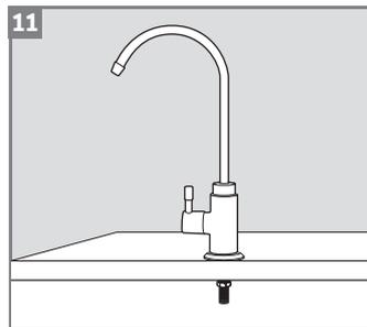
Insert the base washer to the screw beneath the faucet's main body and insert the faucet to the hole.
