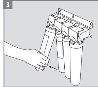
Pull the adapter connector to an angle of 45° while holding the filter.
